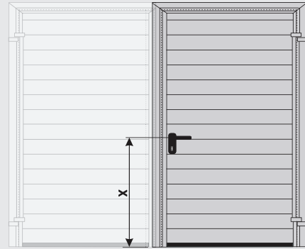
The section height and the height of the handle 'x' depend on the actual door height and construction of the door.
