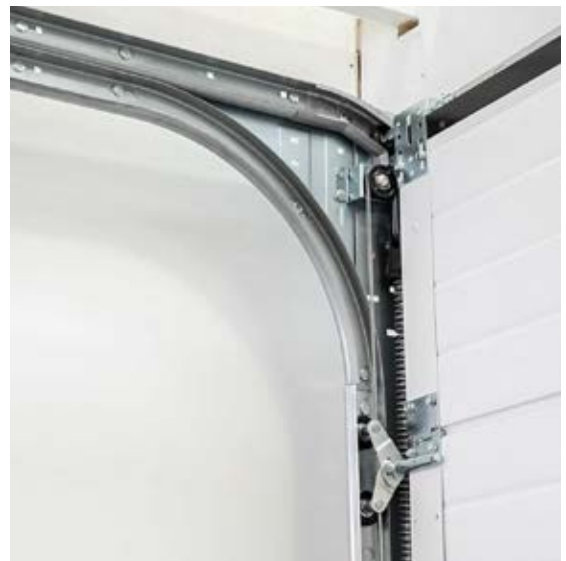
Side extension springs assist the lifting of the door on smooth-running rollers into the overhead tracks.
