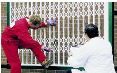
SeceuroGuard 1001 undergoing a simulated attack test.
