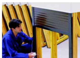
A motorised shutter under test after factory fitting of the shutter to the window frame. Curtains are usually installed on site after the window is installed.
